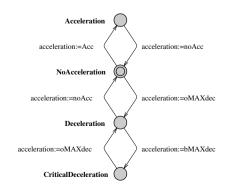
Figure 4-21. Timed automaton model of acceleration sensor
