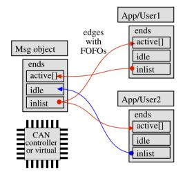
Figure 2-3. LinCAN driver message flow graph edges
