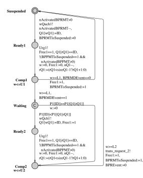
Figure 4-16. Timed automaton model of Task2
