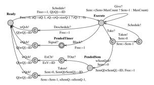
Figure 4-32. Scheduler model containing Take and Give of one semaphore (extension of Figure 4-26)
