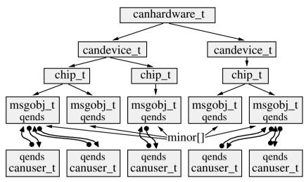
Figure 2-4. CAN hardware model in the LinCAN driver
