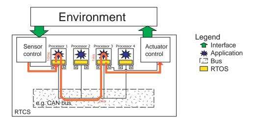
Figure 4-1. Real time control system structure with denotation of computation/communication times
