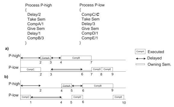
Figure 4-23. Example of monoprocessor scheduling anomaly
