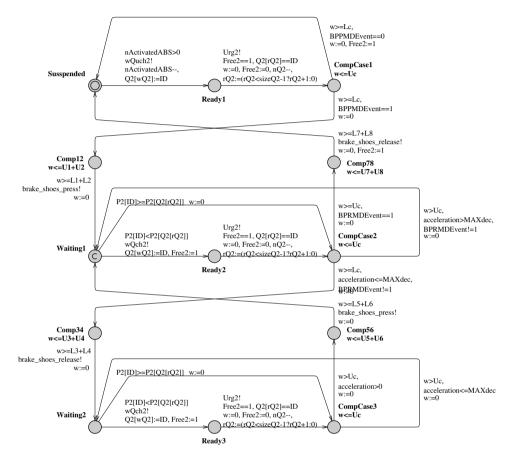
Figure 4-19. Timed automaton model of ABSTask algorithm
