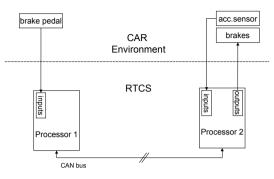
Figure 4-11. Structure of the distributed system - ABS control
