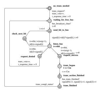
Figure 4-4. Transceiver model
