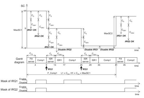
Figure 4-30. Time diagram of ISR execution within interrupt server
