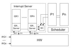
Figure 4-27. System architecture with interrupt server
