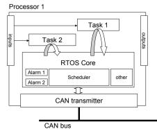
Figure 4-14. Processor 1 structure
