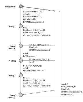
Figure 4-15. Timed automaton model of Task1
