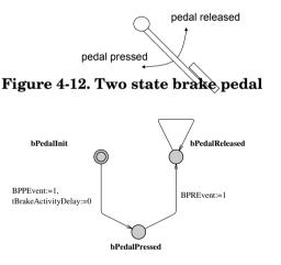
Figure 4-13. Brake pedal model
