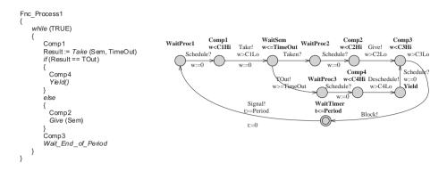
Figure 4-31. Model of process containing Take and Give one semaphore
