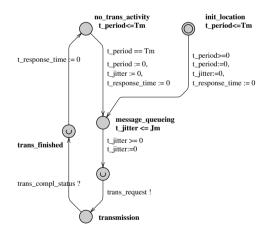
Figure 4-7. Periodic application process model
