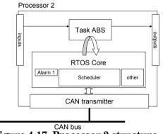
Figure 4-17. Processor 2 structure
