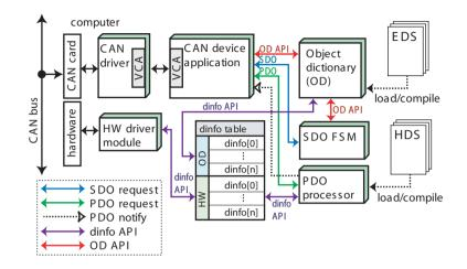
Figure 3-3. RT-CANopen device architecture
