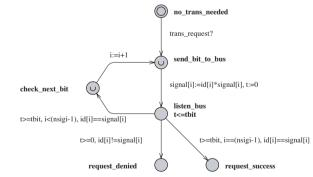
Figure 4-3. Arbitration model (in UPPAAL like notation)
