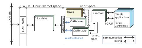
Figure 3-2. Soft real time CAN driver usage example
