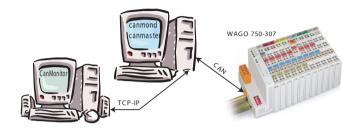
Figure 3-8. CanMonitor testing
